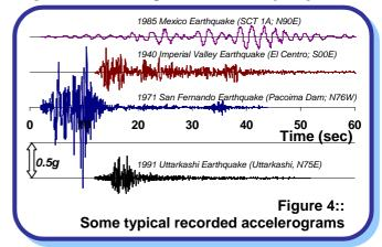
Generally, the maximum amplitudes of horizontal motions in the two orthogonal directions are about the same. However, the maximum amplitude in the vertical direction is usually less than that in the horizontal direction. In design codes, the vertical design acceleration is taken as 1/2 to 2/3 of the horizontal design acceleration. In contrast, the maximum horizontal and vertical ground accelerations *in the vicinity* of the fault rupture do not seem to have such a correlation.
