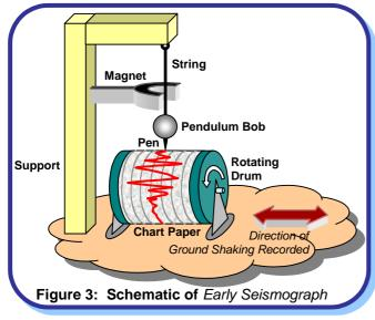
One such instrument is required in each of the two orthogonal horizontal directions. Of course, for measuring vertical oscillations, the *string* pendulum (Figure 3) is replaced with a *spring* pendulum oscillating about a fulcrum. Some instruments do not have a timer device (*i.e.*, the drum holding the chart paper does not rotate). Such instruments provide only the maximum extent (or scope) of motion during the earthquake; for this reason they are called *seismoscopes*.
