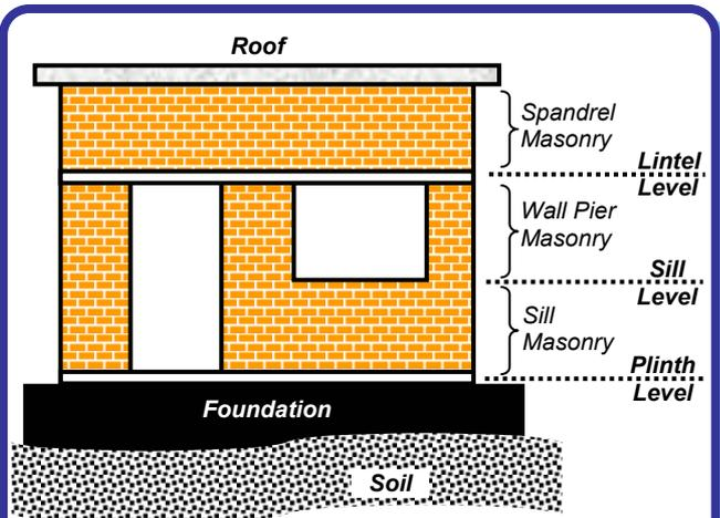
**Figure 1: Sub-units in masonry building – walls behave as discrete units during earthquakes.**
