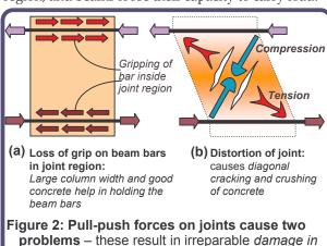
joints under strong seismic shaking.
