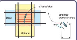
Figure 3: Closed loop steel ties in beam-column joints – such ties with 135° hooks resist the ill effects of distortion of joints.
