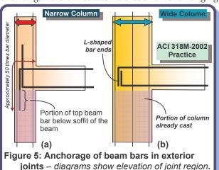
beam top bar in position while casting the column up to the soffit of the beam. On the other hand, if column width is large, the beam bars may not extend below the soffit of the beam (Figure 5b). Thus, it is preferable to have columns with sufficient width. Such an approach has been used in the American practice [ACI318M, 2002].
