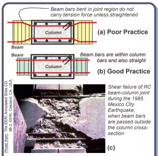
Figure 6: Anchorage of beam bars in interior joints – diagrams (a) and (b) show cross-sectional views in plan of joint region.
