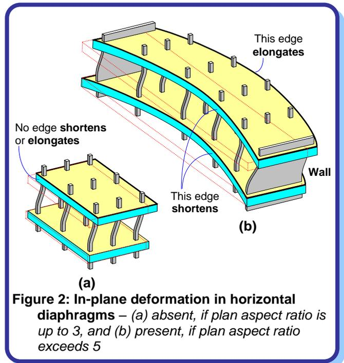
**Figure 2: In-plane deformation in horizontal diaphragms – (a) absent, if plan aspect ratio is up to 3, and (b) present, if plan aspect ratio exceeds 5**
