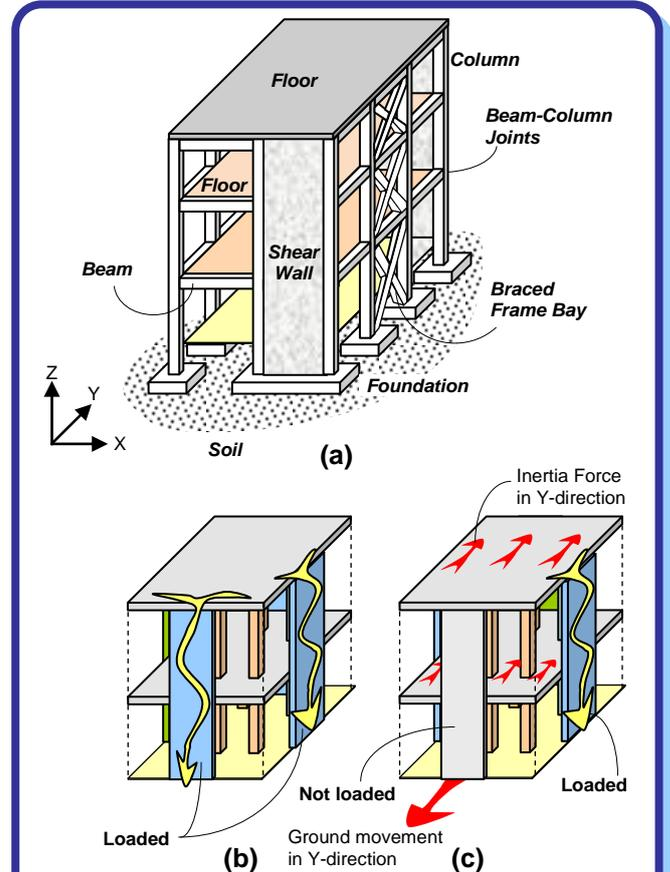
**Figure 1: Load paths for different load actions – (a) key structural elements constituting load paths, (b) vertical load paths, and (c) lateral load paths**
