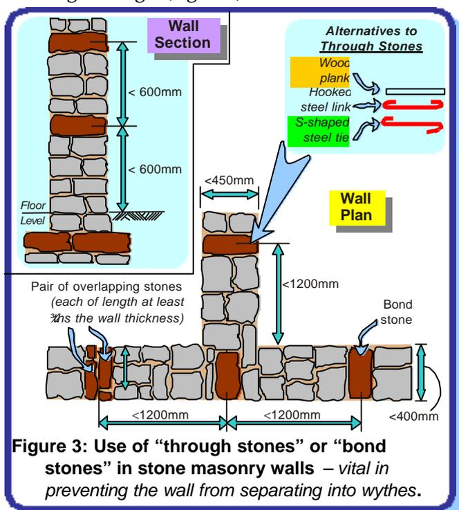
**Figure 3: Use of “through stones” or “bond stones” in stone masonry walls – vital in preventing the wall from separating into wythes.**
