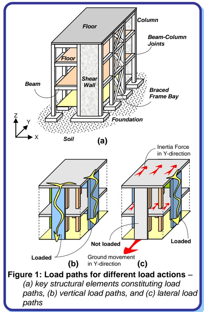
Figure 1: Load paths for different load actions – (a) key structural elements constituting load paths, (b) vertical load paths, and (c) lateral load paths
