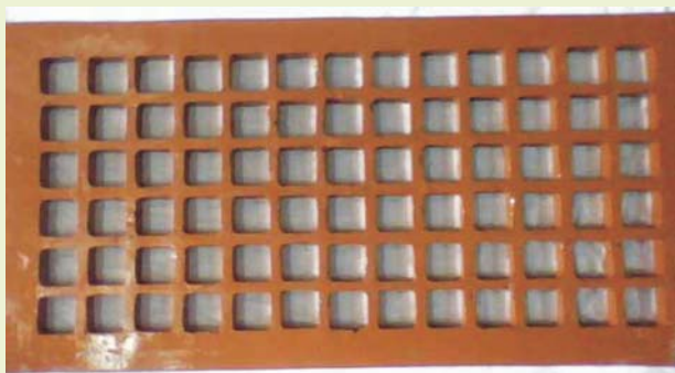
Window from Light wt Natural fibre Polymer composite core
