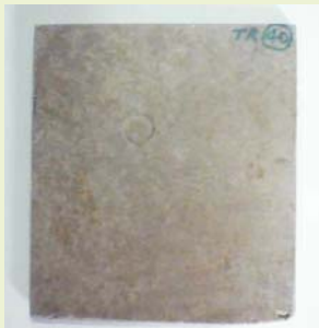
Fig 1a shows the foamed sheet made by Rice husk and polymer (TR40)
