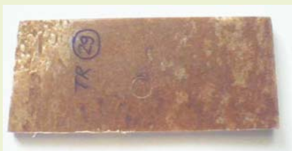
Fig1 d shows the foamed sheet made by Treated RHand another polymer (TR29)
