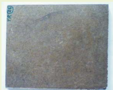
Fig 1c shows the foamed sheet made by rice husk and polymer (TR26)
