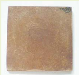
Fig 1b shows the sheet made by treated Bagasse and polymer (TR35)
