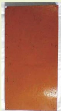
PVC surface covered housing panel from Light wt Nat fib Polymer composite
