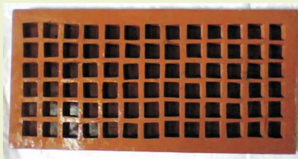
Industrial drainage cover from Light wt Nat fib Polymer composite
