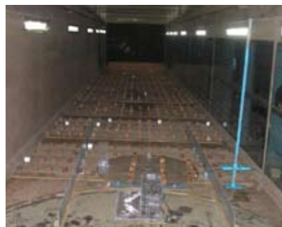
Fig. 4 Cyclone shelter subjected to simulated cyclone wind in wind tunnel
