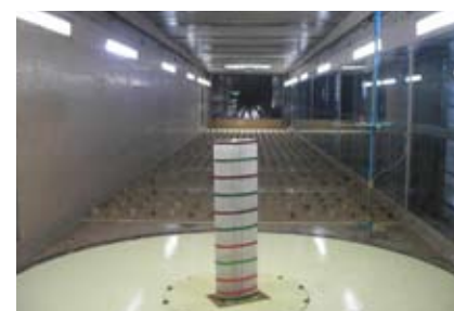
Fig. 5 Model of a Tall Building with Elliptic Plan Shape in Wind Tunnel
