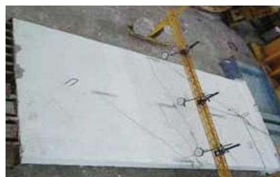
Fig. 5 Light Weight Panels under Axial Compression
