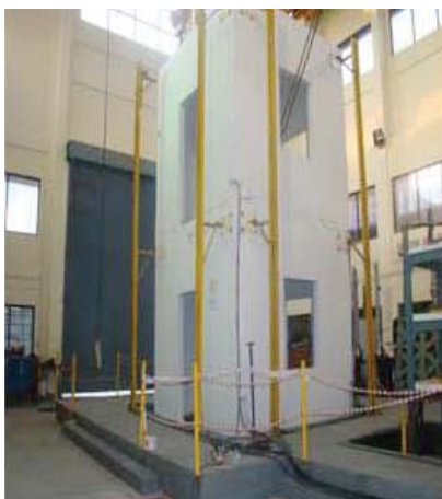
Fig.7 A (G+1) Prefabricated Building assembled on Shake Table for Seismic Test
