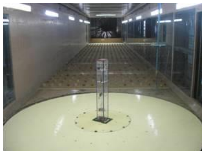
Fig. 2 Model of a Tall Building with Square Plan Shape in Wind Tunnel
