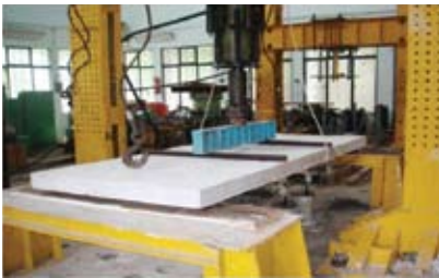
Fig. 3 Flexural Test Set-Up
