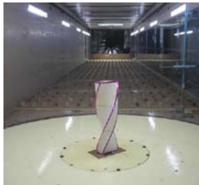
Fig. 6 Model of a Tall Rectangular Twisted Building in Wind Tunnel
