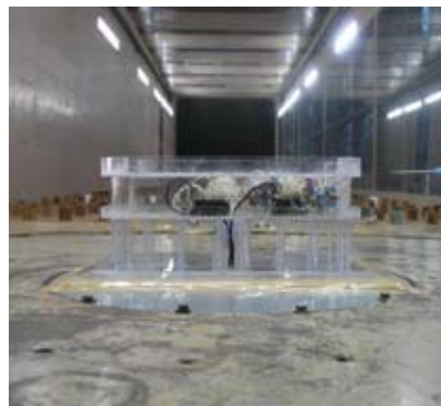
Fig. 3 View of cyclone shelter model in the wind tunnel
