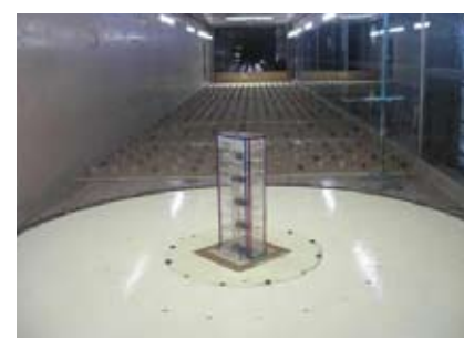
Fig. 4 Model of a Tall Building with Corner-Cut in Wind Tunnel
