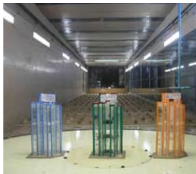
Fig. 7 Models of Group of Tall Buildings in Wind Tunnel
