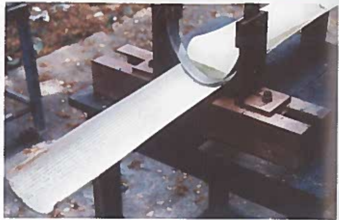
Separation of veneers from the sheath by cleaving
