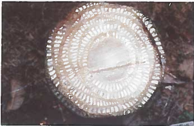
Cross-section of the stem showing concentric layered leaf-sheaths and honeycomb sandwich structure of the sheath
