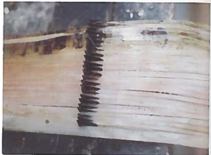
Splitting veneers for preparation of strands
