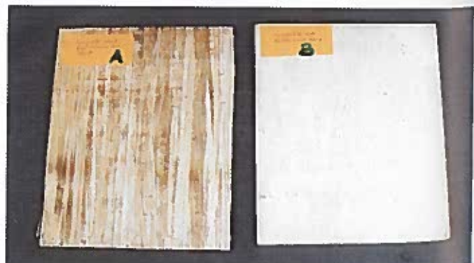
Laminates (A) as obtained from strands and (B) with rubber-wood veneer surface lamination
