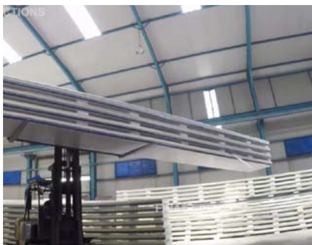
Factory Assembled Insulated Sandwich Panels using PUF
