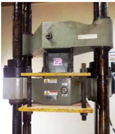
Fig. 3. Experimental Set-up for Pull-out Tests
