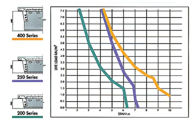
Load span graph – 75mm topping
