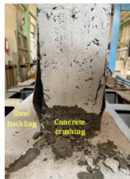
Figure 5 – Failure in the compression side of the shear wall specimen
