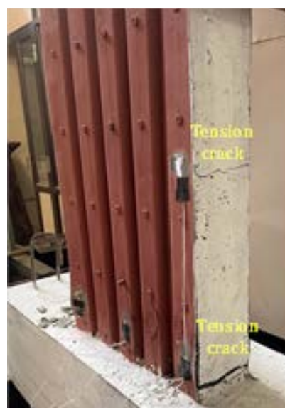
Figure 4 – Failure in the tension side of the shear wall specimen
