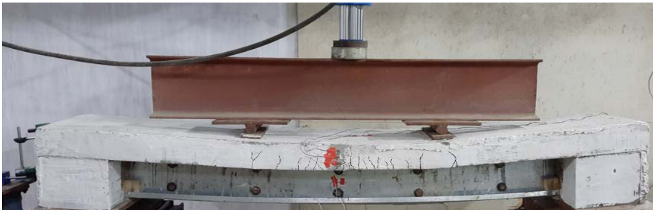
Figure 3 – Failure of Cold-formed steel-concrete composite beam under flexural loading
