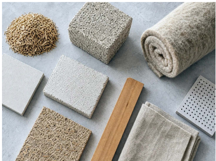
A whole-plant material language: graded shives, hemp-lime, insulation and crafted finishes. Photograph: GoHemp.
