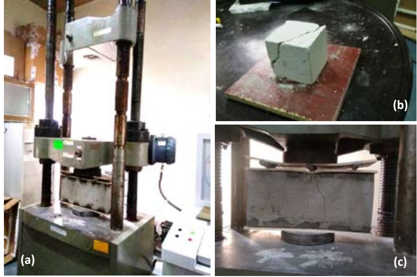
Fig. 2. (a) Compressive strength test set-up; (b) failure pattern of material cube; and (c) failure pattern of FCC block under uni-axial compression
