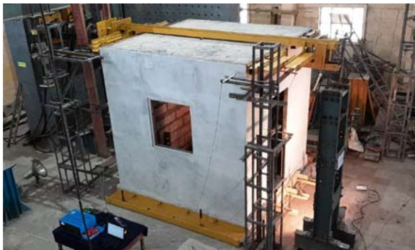
Fig. 4. Experimental set-up for CM building constructed using FCC blocks
