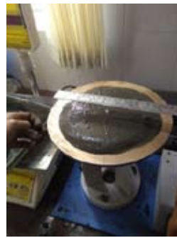
Fig. 5: Flow table test of CBA mortar
