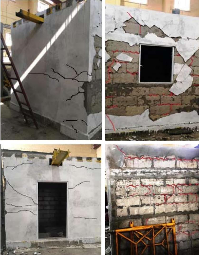
Fig. 5. Damage pattern of tested CM building using FCC blocks
